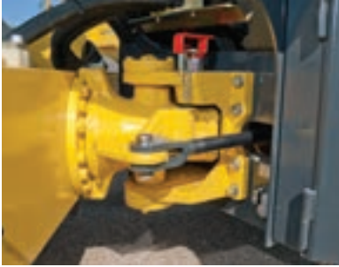
Maintenance-free, rugged, oscillating-articulation joint is bolted on the outside of the front and rear frames.
